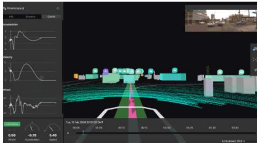
Interface of Uber's Autonomous Visualisation System (AVS) for visualising self-driving vehicles performance. Retrieved from Uber Engineering Blog (UEB, 2019a)
