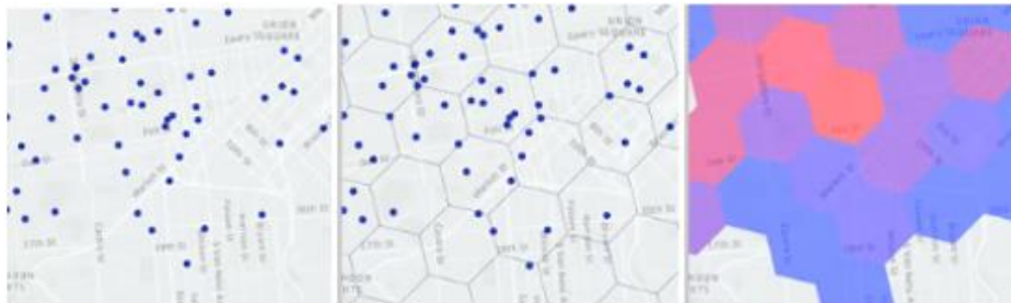
Representation of H3's hexagonal grid layered over a city map. The original caption reads "cars in a city; cars in hexagons; and hexagons shaded by number of cars" (UEB, 2018)
